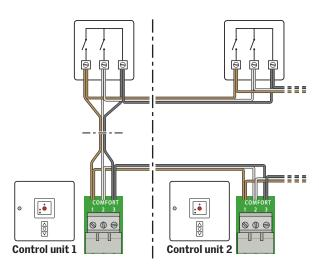
**Note:** Do **not** connect the control systems if you would like a local ventilation switch.
